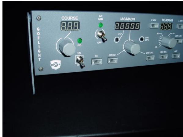
The connection between the MCP and the computer is just one USB cable. I have only tried to plug it directly into my computer and have not found any issues with that. If you e.g. were to use the MCP through a USB-hub I could imagine that it also would work perfectly, however I have discovered that from time to time you can get some strange errors when you use a very complex piece of hardware and run it through a USB-hub, but again I have not tested that with this MCP.
